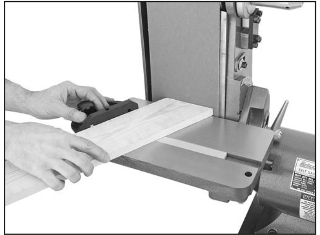
Figure 39. Example of vertical miter sanding.
